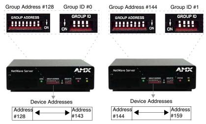
FIG. 2 Relationship between Group Address and Device Address
